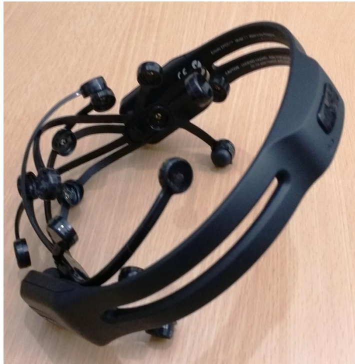
Fig. 1 Commercially available EEG signal acquisition hardware Emotiv EPOC Neuroheadset
