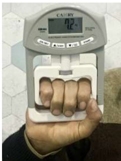
Figure 1: CAMRY® electronic hand dynamometer for grip strength evaluation.
