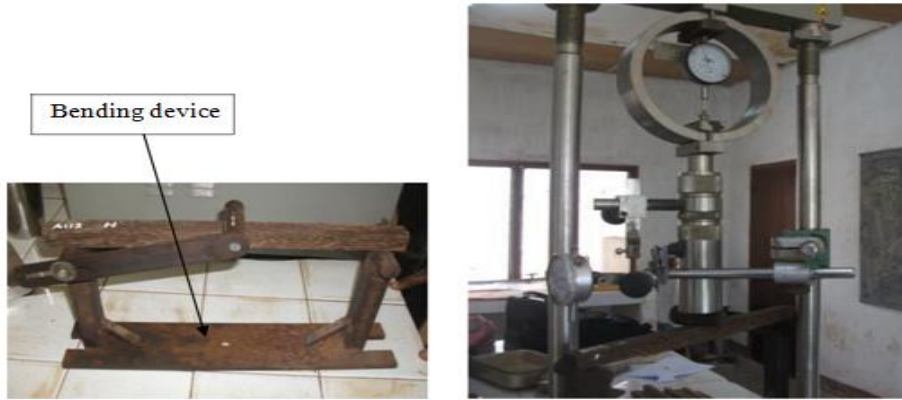
Figure-8: CBR press with bending device
