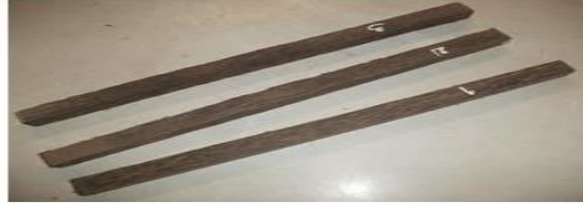
Figure-5: Test rods extracted from slats
