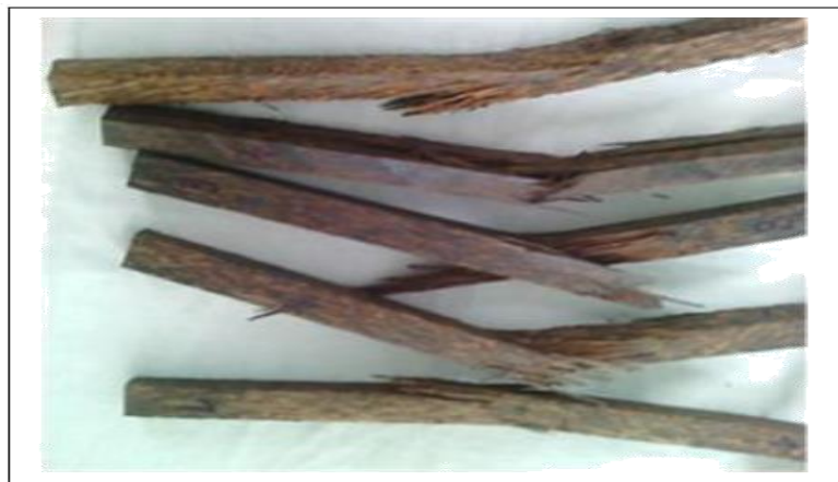
Figure 14:- Form of the sample tested after flexion
