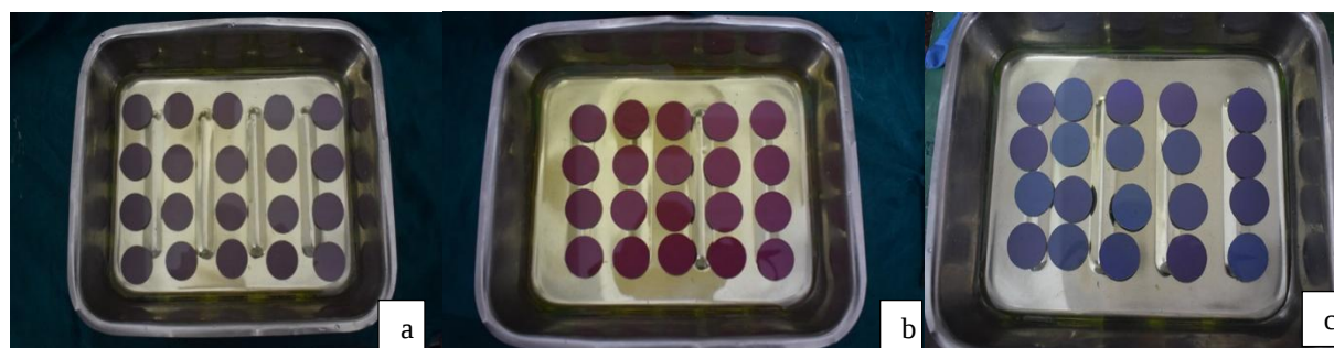
Figure 2:- a) VPES-D, b) PVS-D, c) PE-D samples in disinfection solution.
