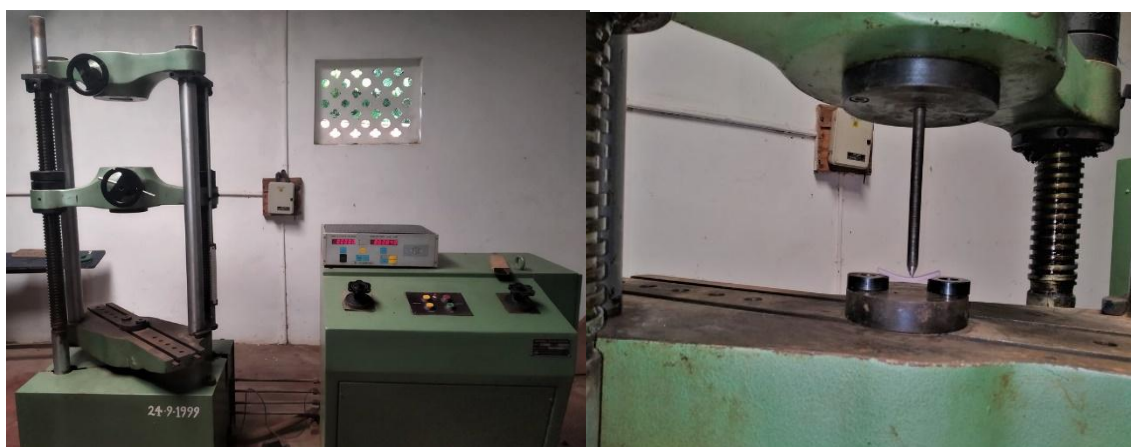
Fig 11:- Universal Testing Machine Fig 12: Load applied in the center of the specimen
