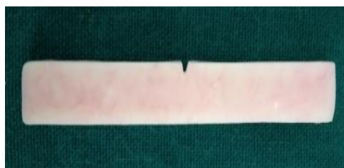
Fig 8:- 'V' shaped notch made at the center for impact strength test.
