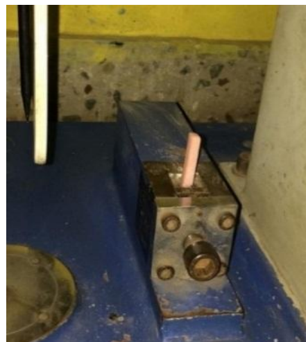
Fig 10:-Specimen placed vertically in Impact tester (Izod method).
