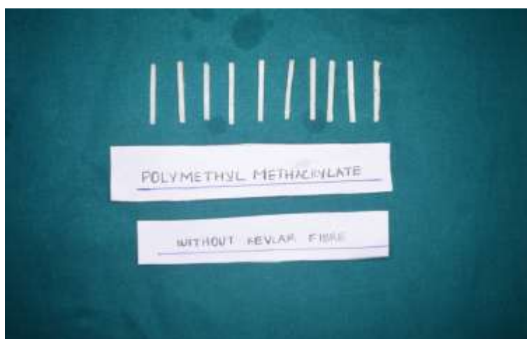
Figure 10:- Polymethyl methacrylate without Kevlar fibre (Flexural strength).
