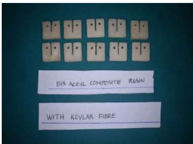
Figure 9:- Bisacryl composite with Kevlar fibre (Fracture toughness).
