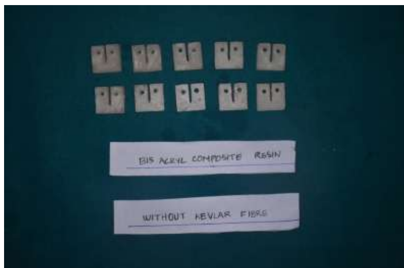
Figure 7:- Bisacryl composite without Kevlar fibre (Fracture toughness).
