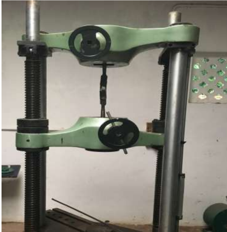
Figure 14:- Samples subjected to fracture toughness on universal testing machine.
