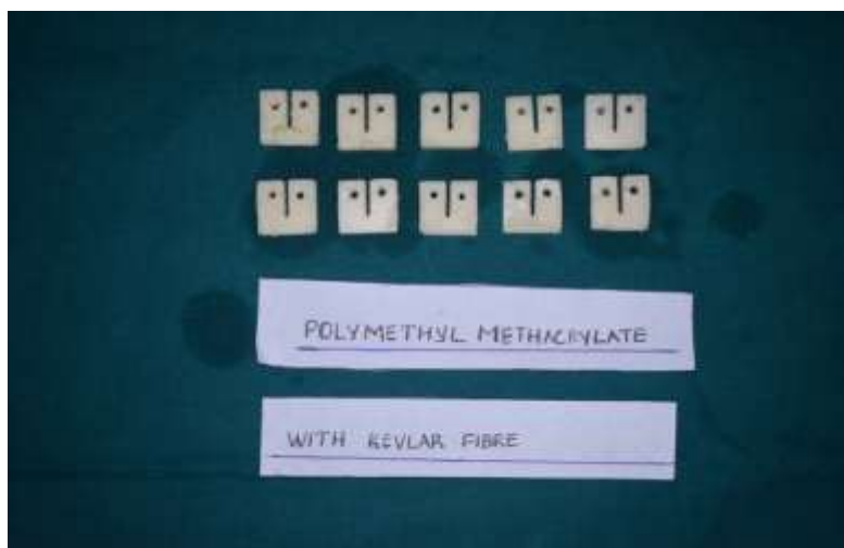
Figure 8:- Polymethyl methacrylate with Kevlar fibre (Fracture toughness).
