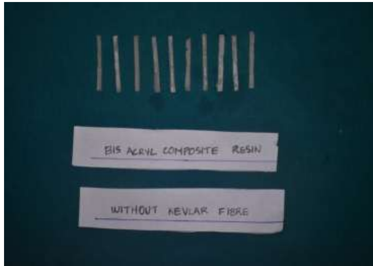
Figure 11:- Bisacryl composite without Kevlar fibre (Flexural strength).
