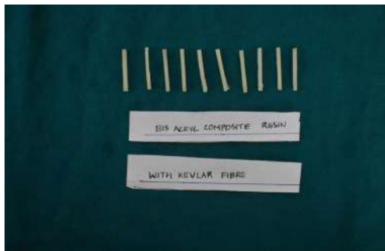
Figure 13:- Bisacryl composite with Kevlar fibre (Flexural strength).
