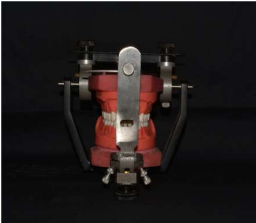
Figure 5:- Positioning jig attached to the incisal pin portion of the Hanau Wide Veu articulator.
