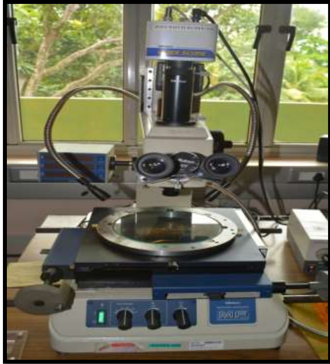
Figure 4:- Toolmakers Measuring Microscope, (MITUTOYO, Japan) used for the measurement of dies.
