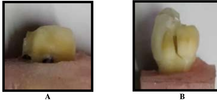
Figure 2:- A- Complete debonding of the endocrown without fracture of the tooth (favourable failure), B- Fracture of the endocrown/tooth complex (catastrophic failure)
