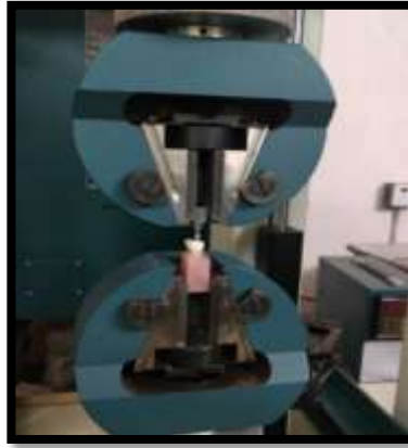
Figure 1:- Mounted tooth placed in universal testing machine with stainless steel ball attached.
