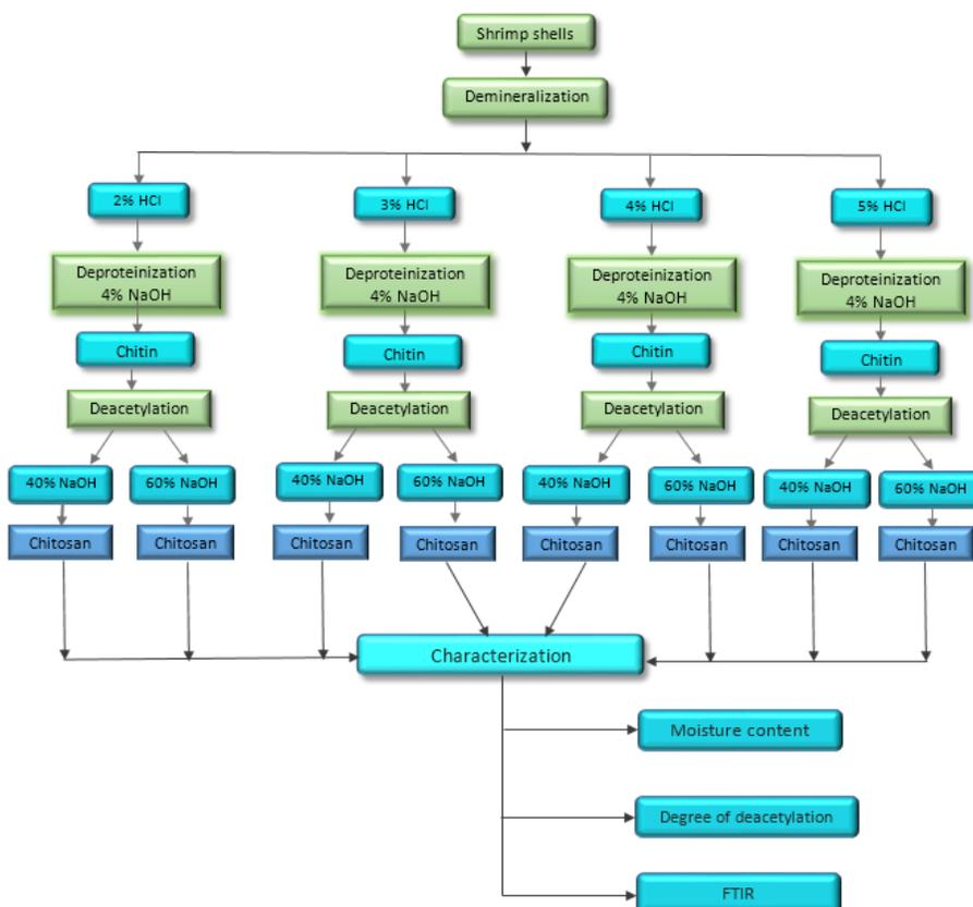
Figure 2: Schematic diagram of chitosan extraction
