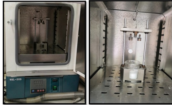
Fig.5 Dip coater device and specimen during coating.
