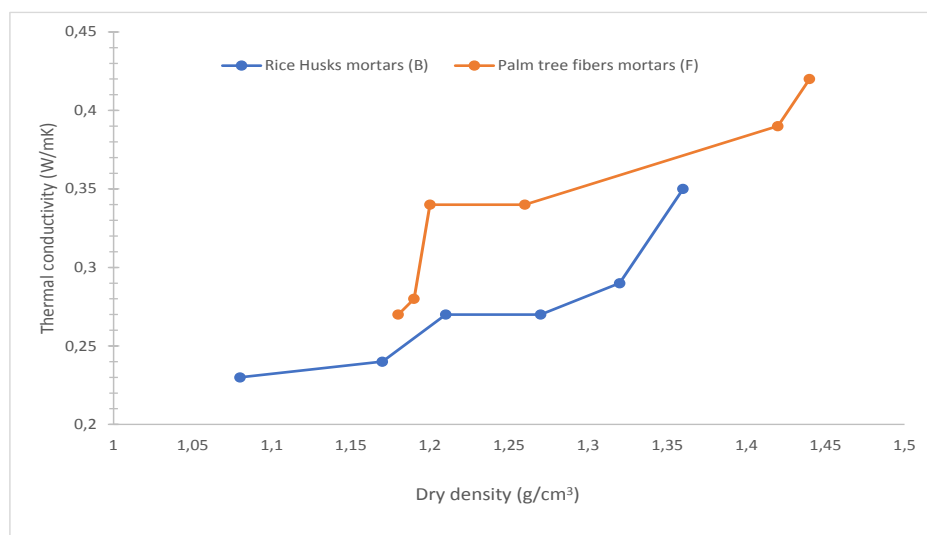
Figure 4:- Thermal conductivity vs dry density of studied specimens.
