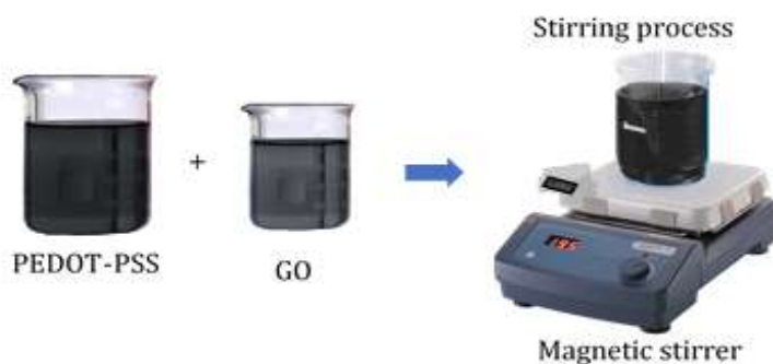
Figure 1:- Stirring process of PEDOT:PSS and GO.
