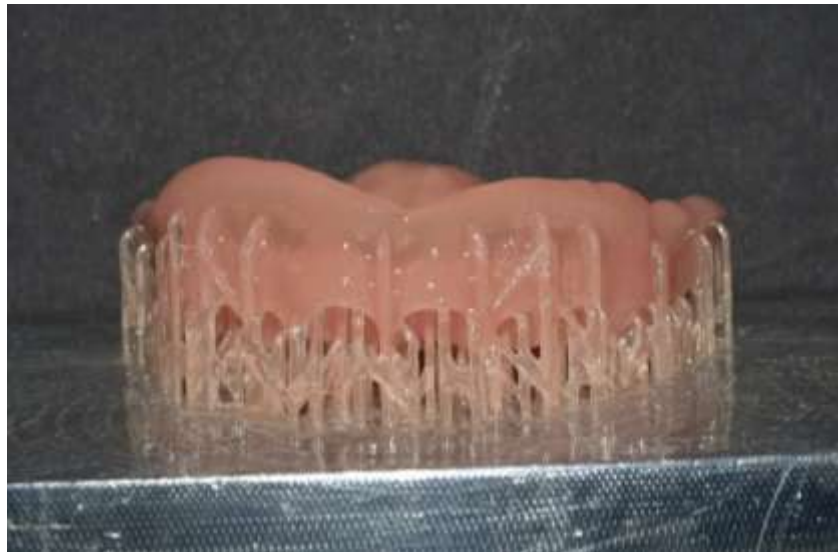
Figure (5):- 3D printed denture bases denture bases.
