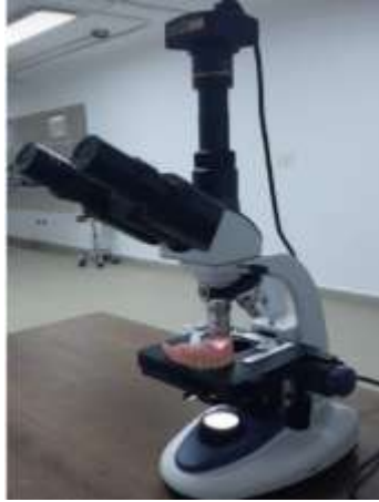
Figure (6):- Digital microscope with a built-in camera.
