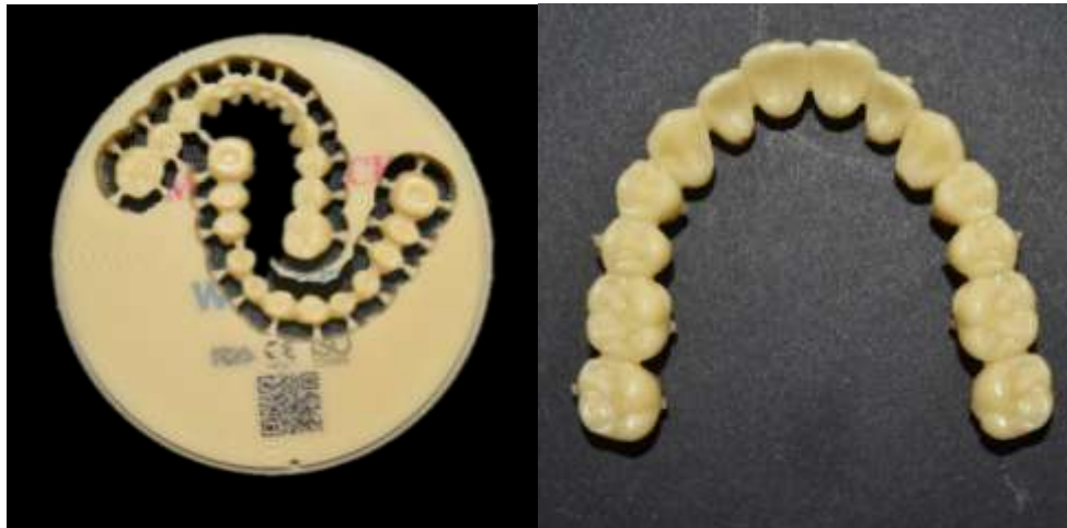
Figure (3):- Milled upper and lower set of teeth.
