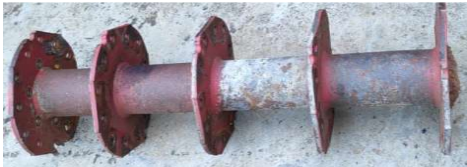
Figure 3:- Breakdown in rotor shaft (factory-site captured picture).
