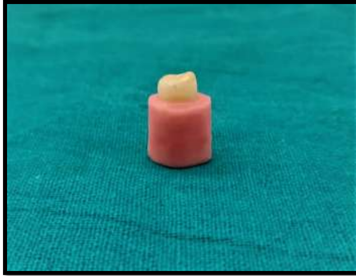
Fig1:- Acrylic mounting of tooth.
