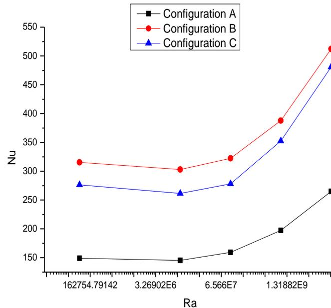
**Figure 11:-** Comparison of the influence of Rayleigh number on the Nusselt number of the thermosiphon and the thermosiphon with a heating source for the three configurations.
