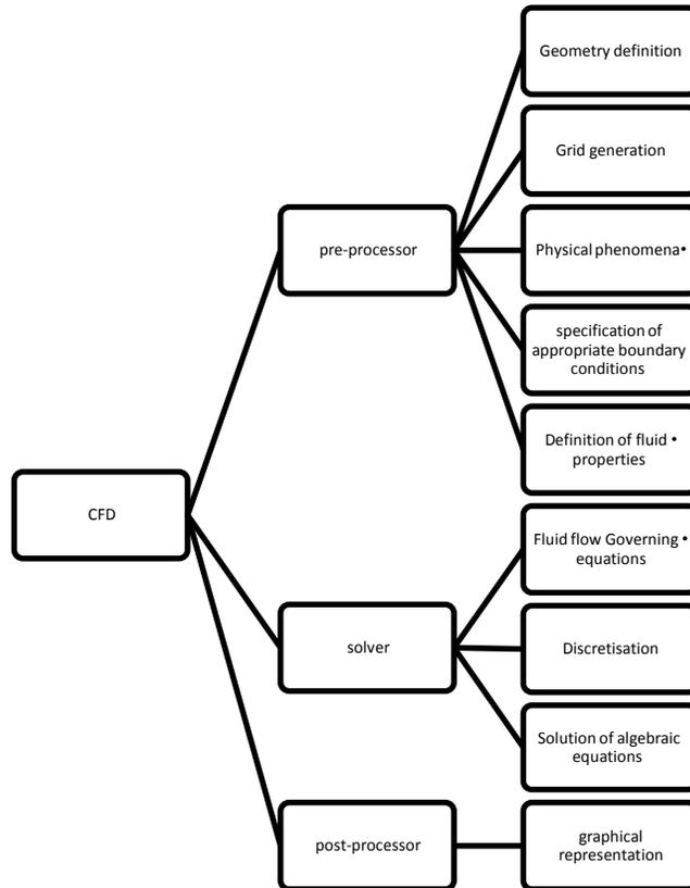
Figure 1:- CFD Analysis Process.
