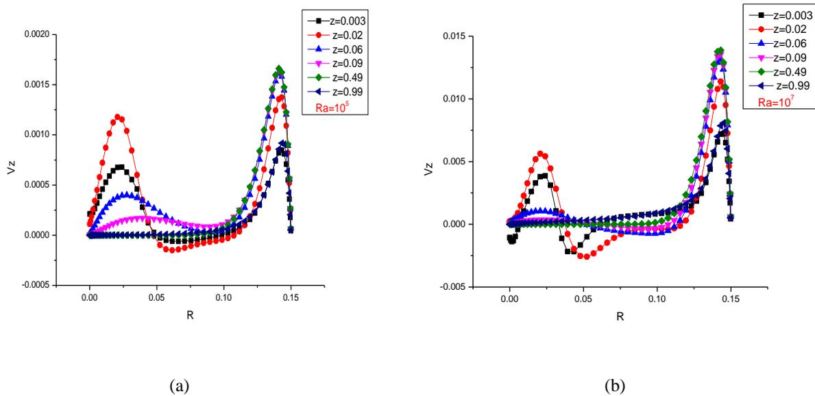
Figure 5 (a,b):- Radial evolution of the vertical dimensionless velocity at different levels Z of Rayleigh number at (a) $10^5$  and (b) $10^7$ .
