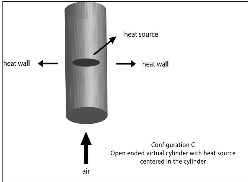
Figure 4:- Open-ended vertical cylinder with a heat source centered in the cylinder (zs = 0.04).
