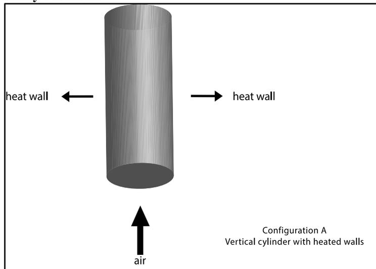
Figure 2:- Vertical channel with heated walls.
