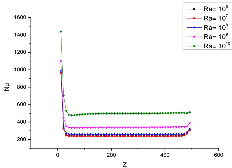
**Figure 7:-** Axial evolution of Nusselt number at different values of Rayleigh.
