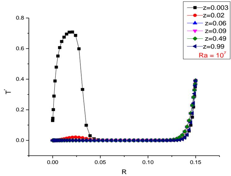
**Figure 6:-** Radial evolution of the dimensionless temperature at different levels Z of Rayleigh number at  $10^7$
