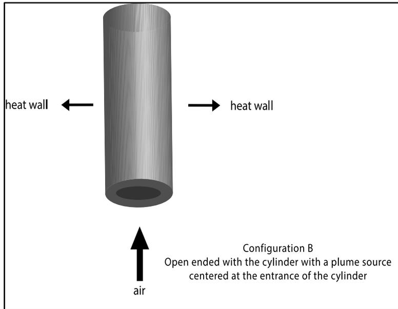
**Figure 3:-** Open-ended vertical cylinder with a plume source centered at the cylinder inlet.
