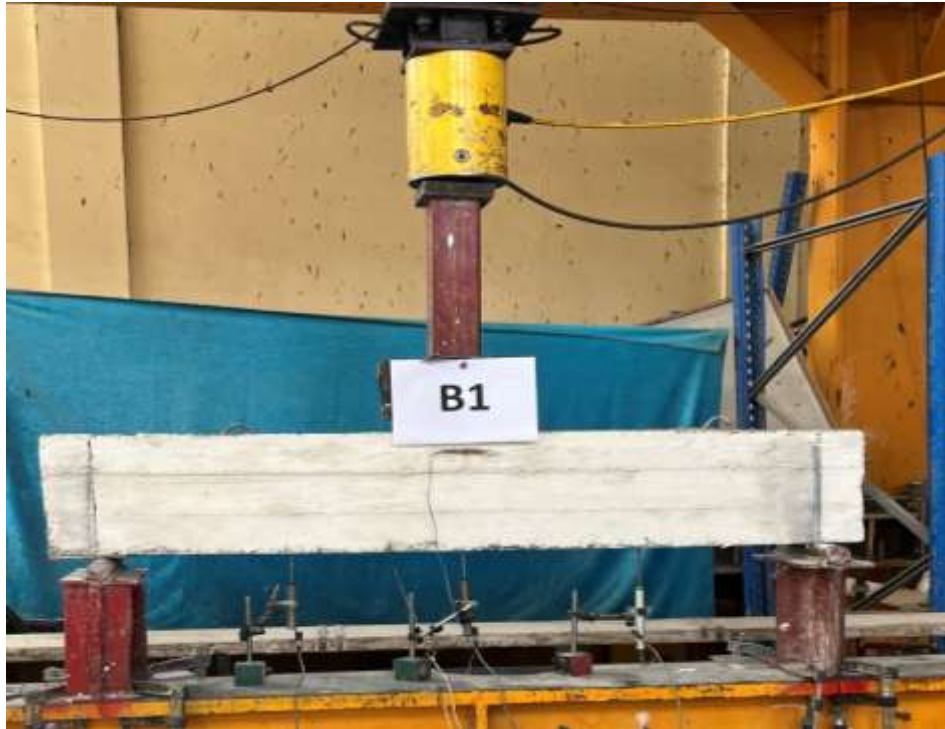
Fig. 5:- Test Setup for Specimens during Loading.
