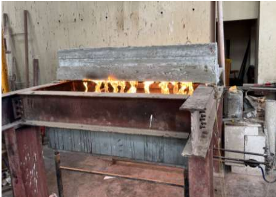
Fig. 6:- Test Setup for Specimens during Fire.
