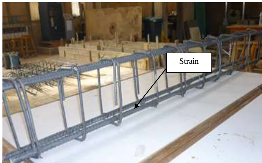
Fig. 4:- Steel Mesh of Rectangular Beams.
