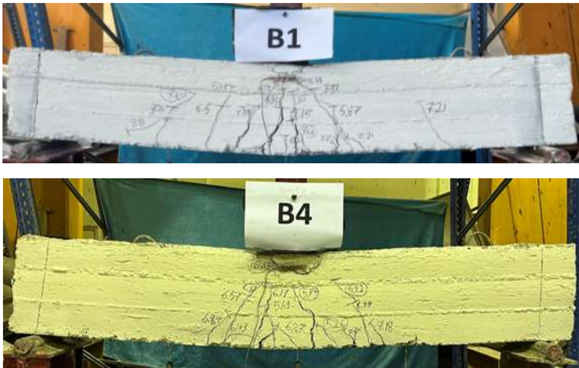
Fig. 9:- The Crack Patterns for B1(NNC) and B4(FNC).
