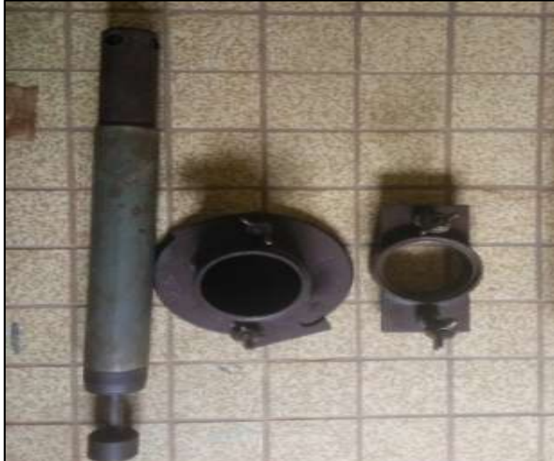
Figure 5:- Small proctor hammer, mold and collar (from left to right).
