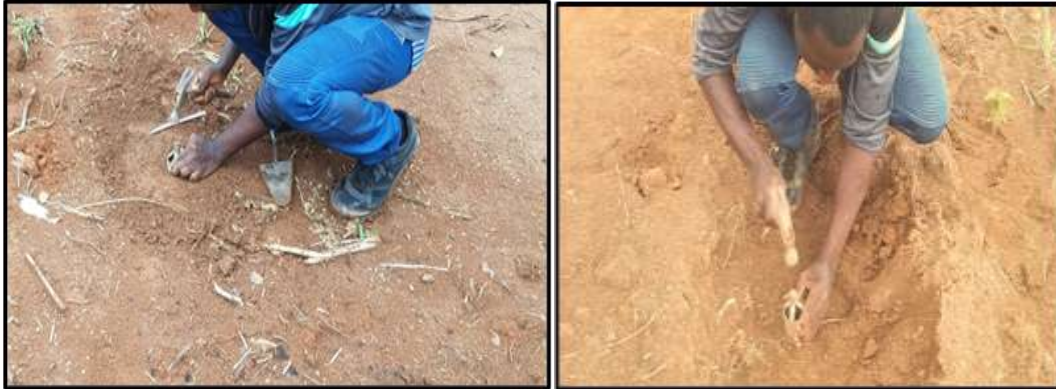
Figure 3:- Core ring being hammered into the soil at 0-15cm and 15-40 cm depth.
