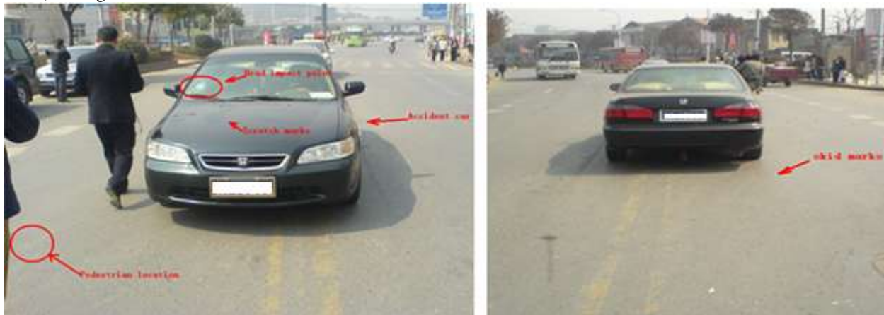
Figure 1:- Impact locations of the male pedestrian on the Honda Accord 2001 model.
