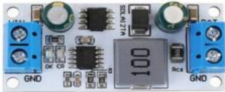
Figure 14:- Battery charger module.
