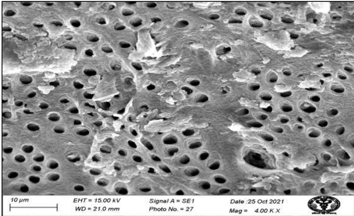
**Fig 3:-** Sem Photomicrograph Of A Specimen Treated With 25% Tetracycline Hydrochloride (Magnification 4000X).
