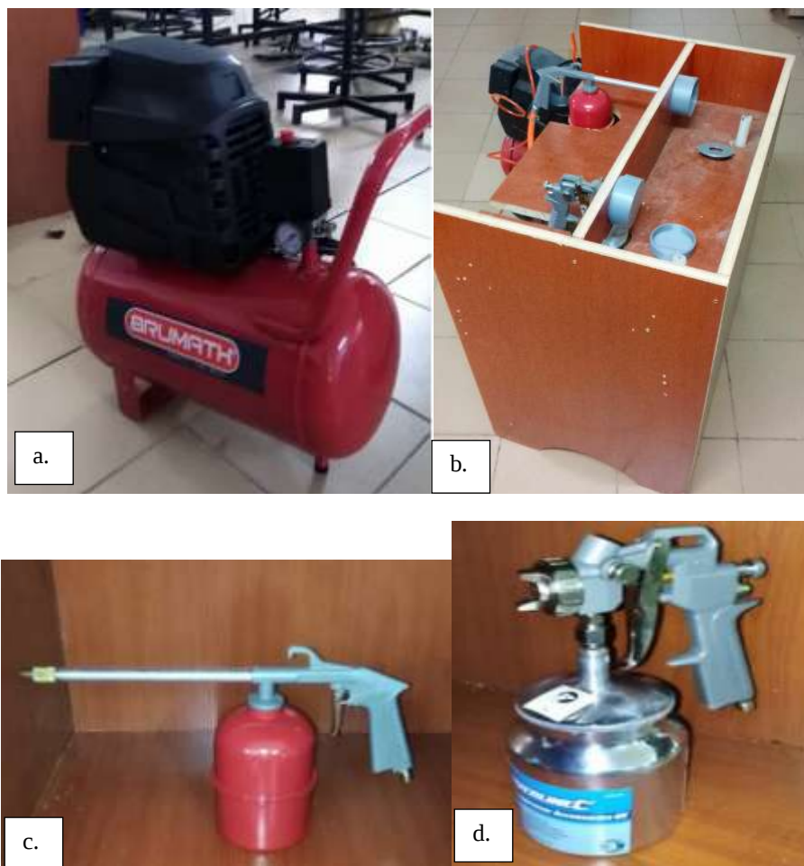
a. Compressor ; b. Complete control bench ; c. Blower ; d. Spray Figure 2:- The control bench and its components.
