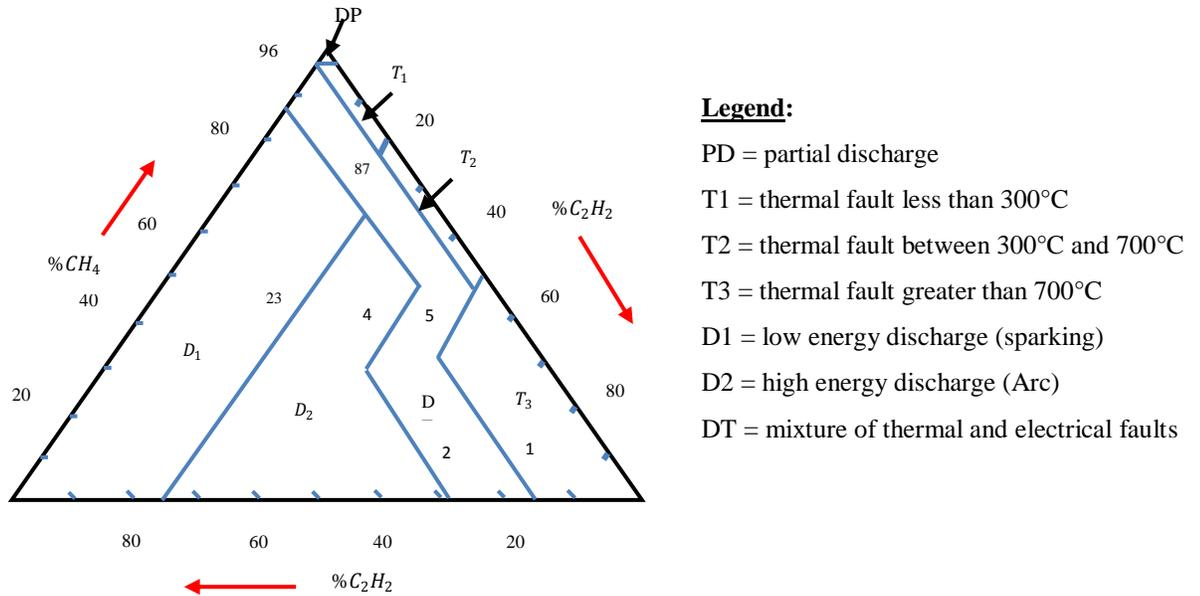
Figure 1:- Diagram of Duval's triangle [26].
