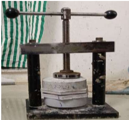
Fig. 7:- CPVC pipe with mechanical press.
