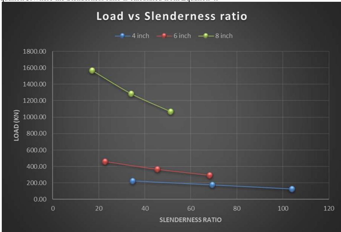
Fig 17:- Load vs. Slenderness ratio of TDGLC with different cross-sections.
