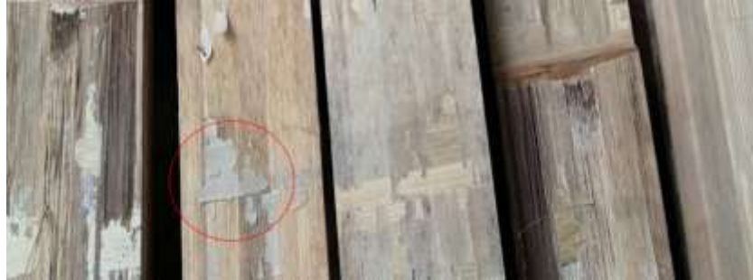
Figure 7:- Splitting Mode cause by glue failure.
