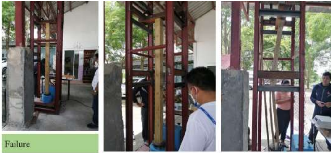
Fig. 11:- Buckling Failure MODE II.
