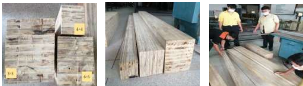
Figure 4:- The TDG column is a. cross-section, b. length, and c. cut to various lengths.
