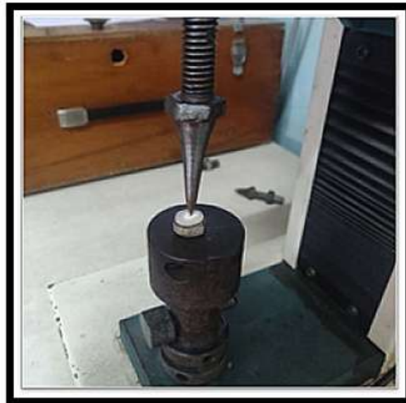
Figure 3:- Push-Out Bond Strength Using Universal Testing Machine.
