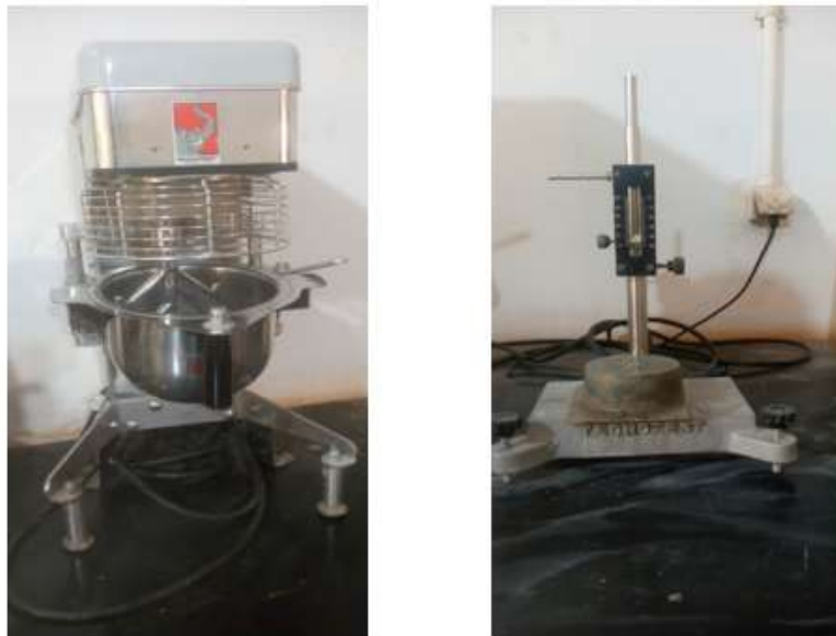
Figure1:- a. TECNOTEST mixer, b. Vicat equipment.
