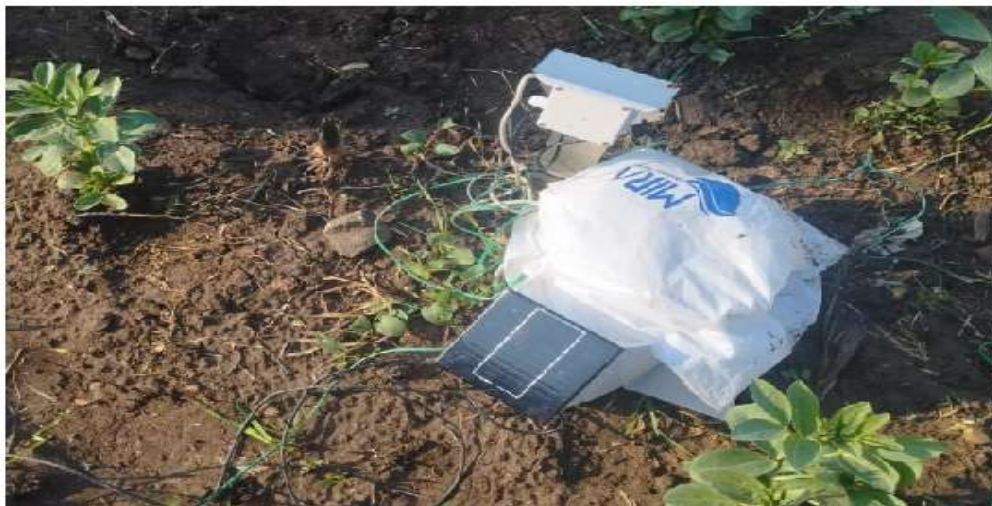
Fig. (1) The device for measuring soil water tension with three watermark sensors.
