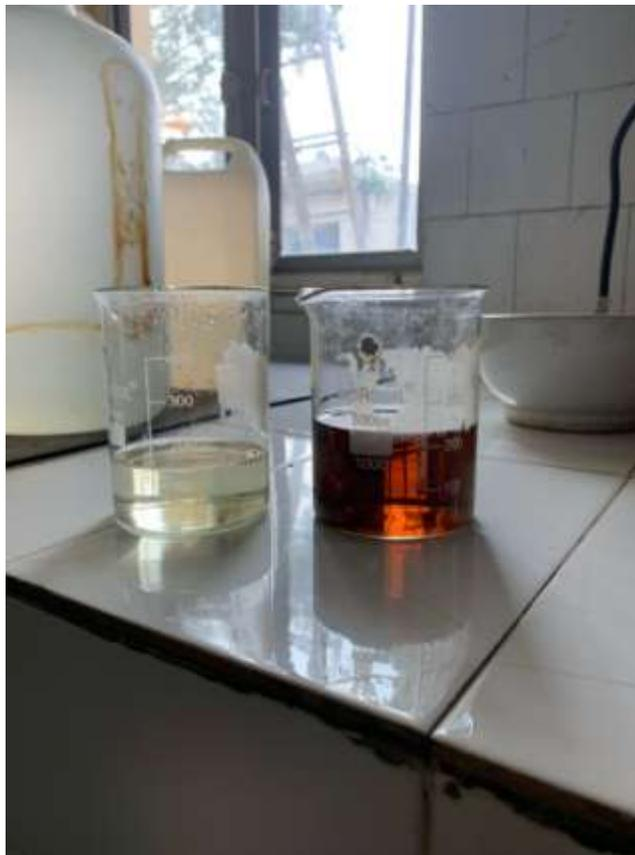
**Fig.2:-** Visual Comparison of waste and lab recovered Sulphuric acid.
