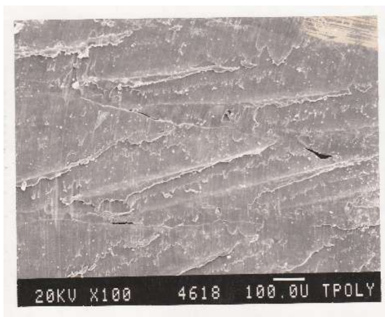
Fig 2:- Stainless steel 18-9 treated under H 2 till 750°C.
