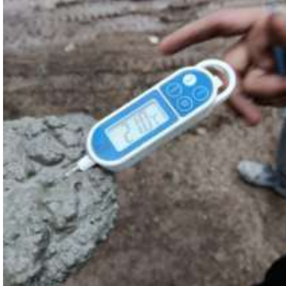
Figure 4:- Temperature of Concrete Maintained below 25 Degree Celsius.
