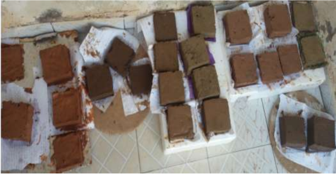
Fig 1:- Molded building blocks undergoing drying process.
