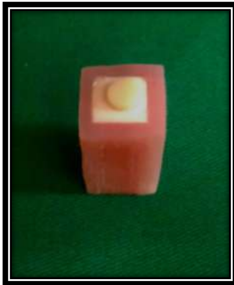
Figure 6:- Composite rod placed on zirconia specimen using resin cement
