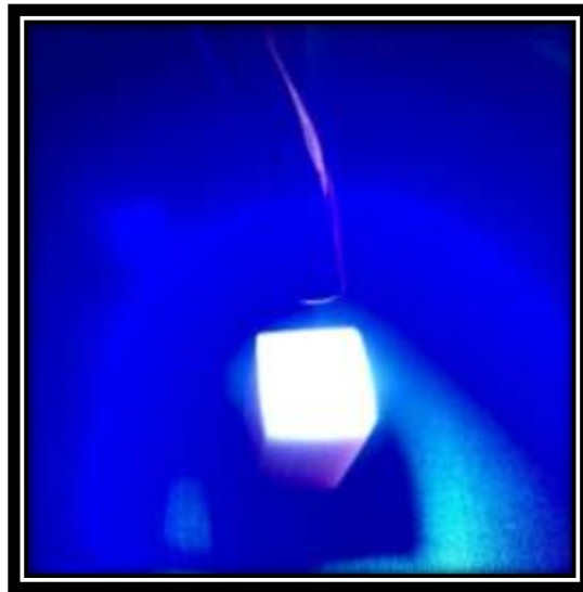
Figure 7:- Light curing of composite rod to zirconia specimen.
