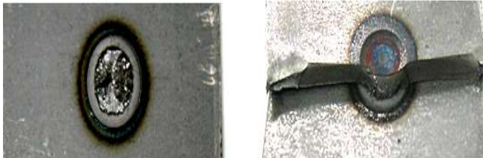
(a) Shear failure of the nugget
