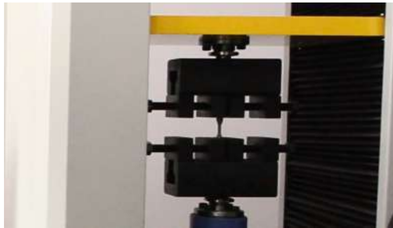
Fig 2 :Fatigue Test conducted using computerized fatigue machine
