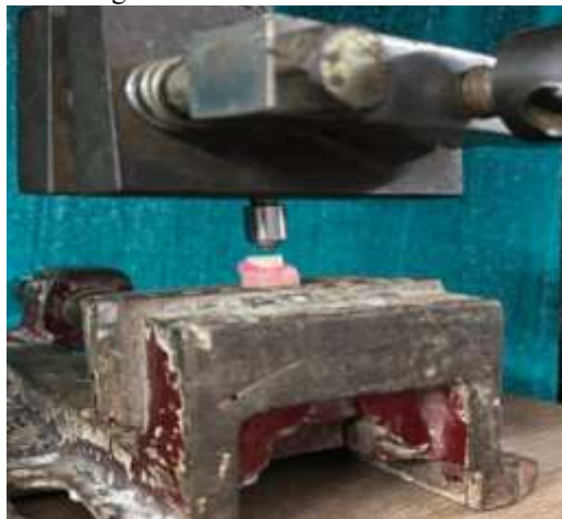
FIGURE 2- SAMPLE MOUNTED ON UNIVERSAL TESTING MACHINE
