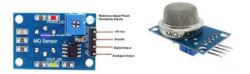
The Module requires a 5V power supply and provides a digital Logic output (1 or 0) and an analog level output (0-4V). The digital logic output is LOW (0) when no gas is detected but goes HIGH (1) when hazardous gas concentration in the environment reaches the set threshold set via a potentiometer on the module.
