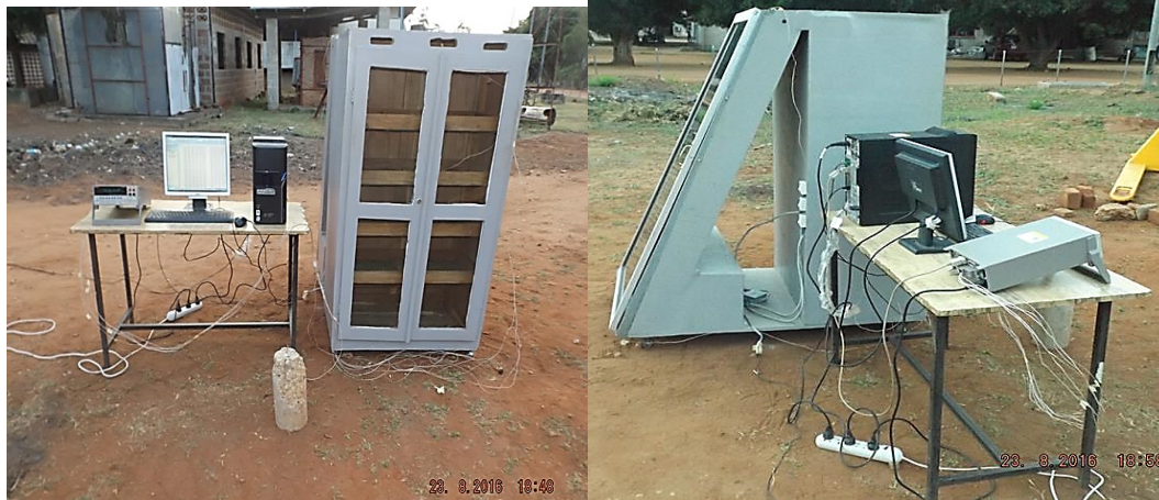
Figure 2 : Instrumentalized indirect solar dryer for temperature measurements.
