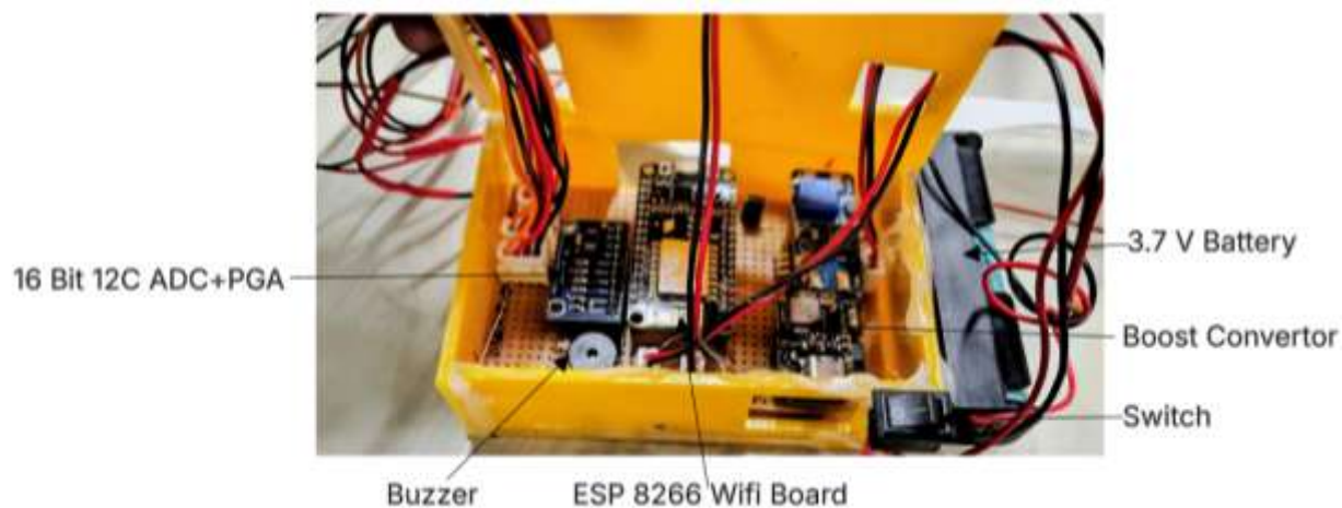
Figure 2: Circuit Board with ESP8266
