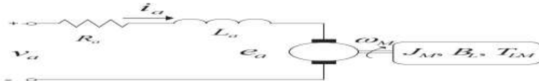
Figure 3: CC motor equivalent circuit
