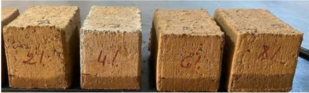
Figure4: Composite samples after capillary absorption testing
