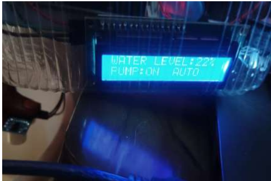
Figure 2. LCD display indicating water level percentage and pump status.
