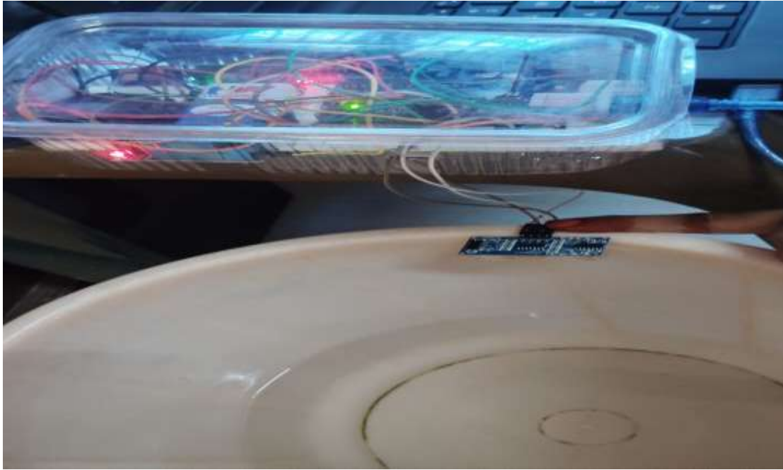
Figure 1. Prototype configuration of the water level monitoring and control system.
