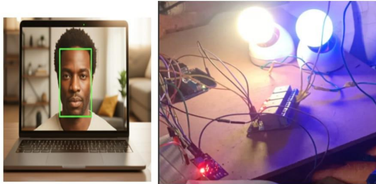
Fig. 7: AI Detection State: Human detected, AI-controlled light ON.
