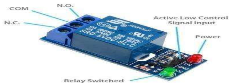
Fig. 4. Single-channel relay circuit for automated pump control
