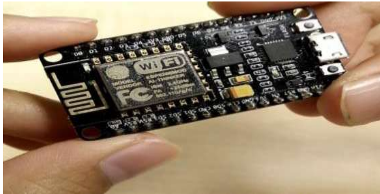
Fig. 6. NodeMCU Wi-Fi module interfaced for cloud data transfer
