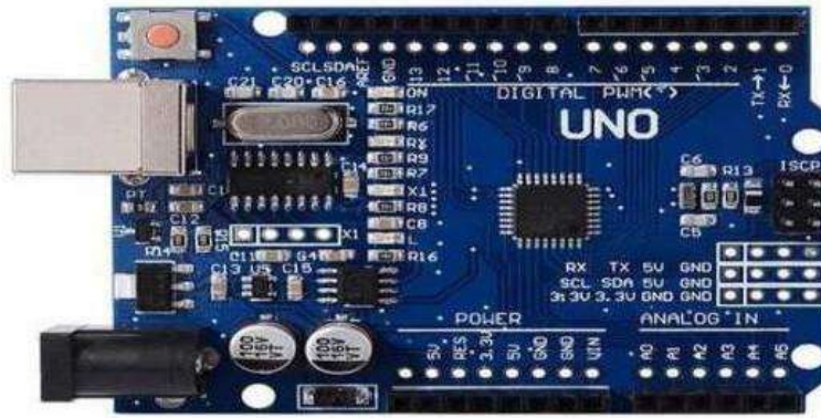
Fig. 3. Arduino UNO microcontroller board used as the central control unit
