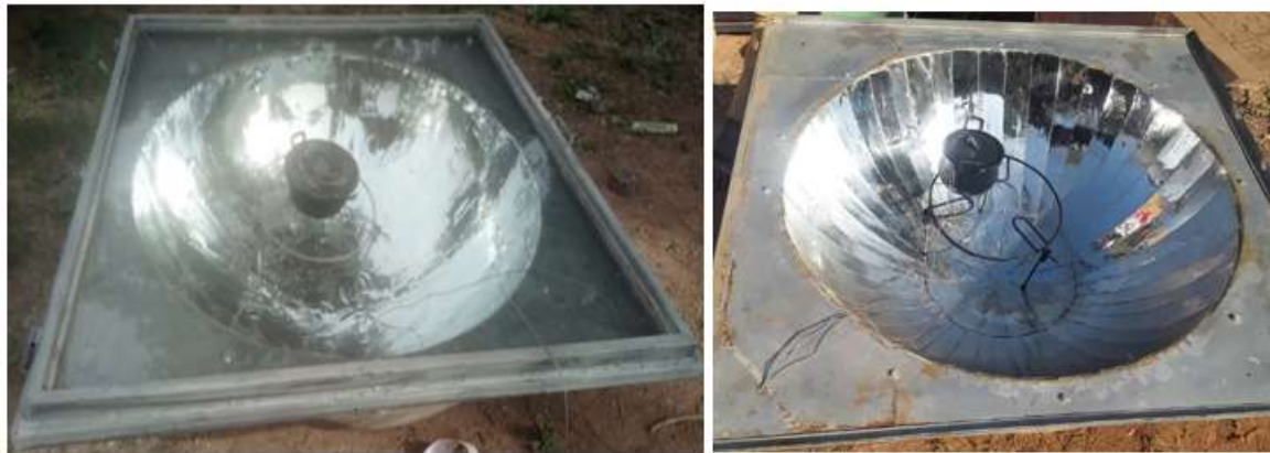
Figure 1: Measuring equipment, experimental setup with and without glazing
