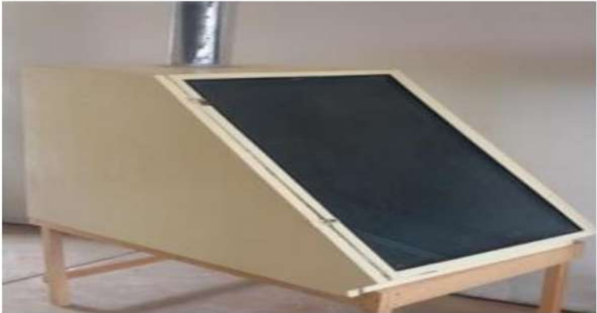
Figure 2. Indirect Natural Convection Solar Dryer
