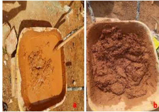
Figure 7: a- Mixture before adding cattail and grass; b- Mixture after adding cattail and grass
