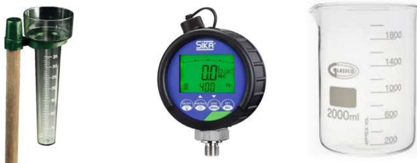
Figure 4: Monitoring device for rainfall, pressure, and dripper water volume
