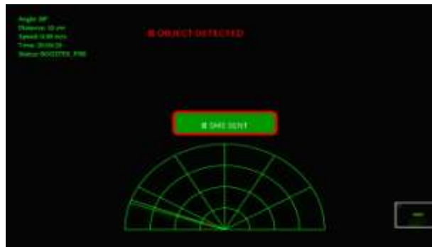
Fig.11. System detecting an object and activating the alert mechanism.
