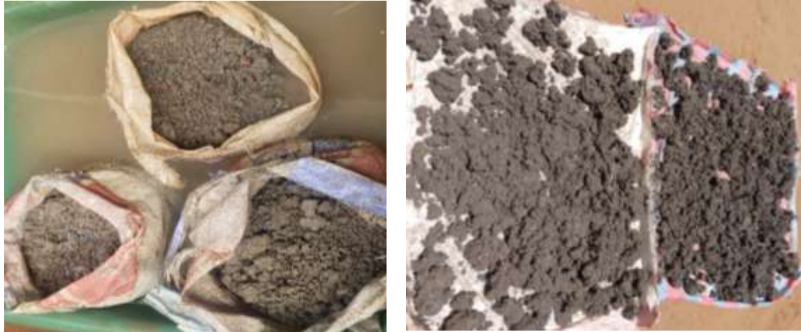
Photo 1: Illustration of the texture of samples that have undergone humidification-drying cycles After each drying cycle, the material is ground in a metal mold and sieved through a 5 mm sieve. The sieve passages are then used to determine the moisture content of the ground material, in order to perform the CBR test.
